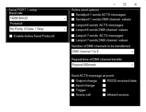
A checkbox to activate ACTS with serial port 1 is available at the Serial port 1 setup area.
