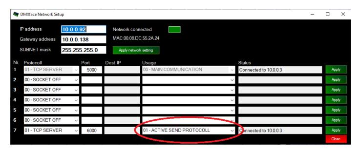
The sockets you want to use for the ACTIVE Send communication must be set to the operating mode ACTIVE SEND PROTOCOL.
